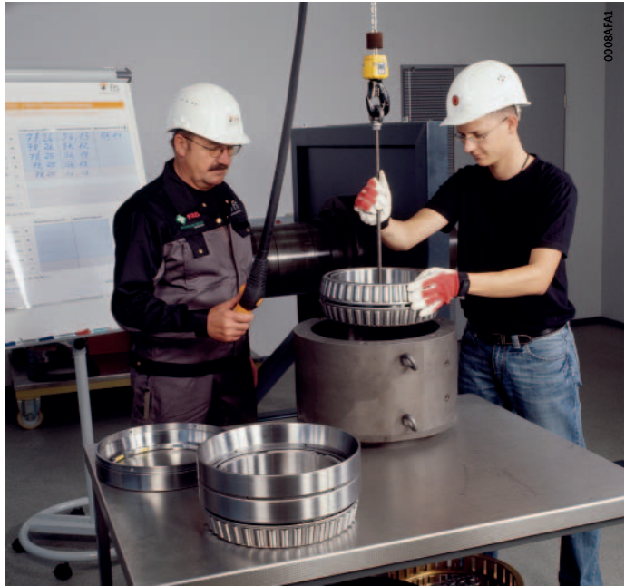
Figure 6 Training course on mounting of rolling bearings
